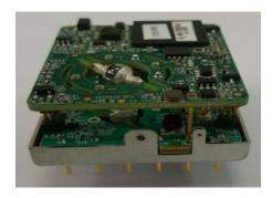
Phase noise (floor): -150dBc / Hz Stability: 1E-10 @ 1s; 8E-12 @ 1000s Power Consumption: < 1.2W Size: 32cc (41.1mm X 35.3mm X 22 mm)
